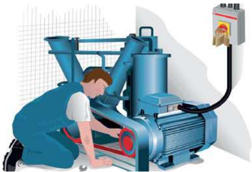
Safety switches protect the operator from unexpected start-up
